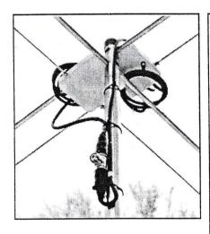
Left photo indicates proper method of dressing phasing line and connector. Note the "A" block (yellow lead) makes a high loop above the antenna, and descends the mast between the driven elements. The "B" block (red lead) loops away from the mast, and then joins the mast just above the T connector. Use 3 ty-wraps as shown to hold assembly in place. Use 2 additional ty-raps to secure your feed line. Waterproof the connection with tape, or Coax-Seal.
